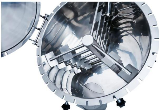
*The mixing rotor of the new bulk mixer MIX-A-LOT ensures a combination of excellent homogenization and shortest mixing time*
